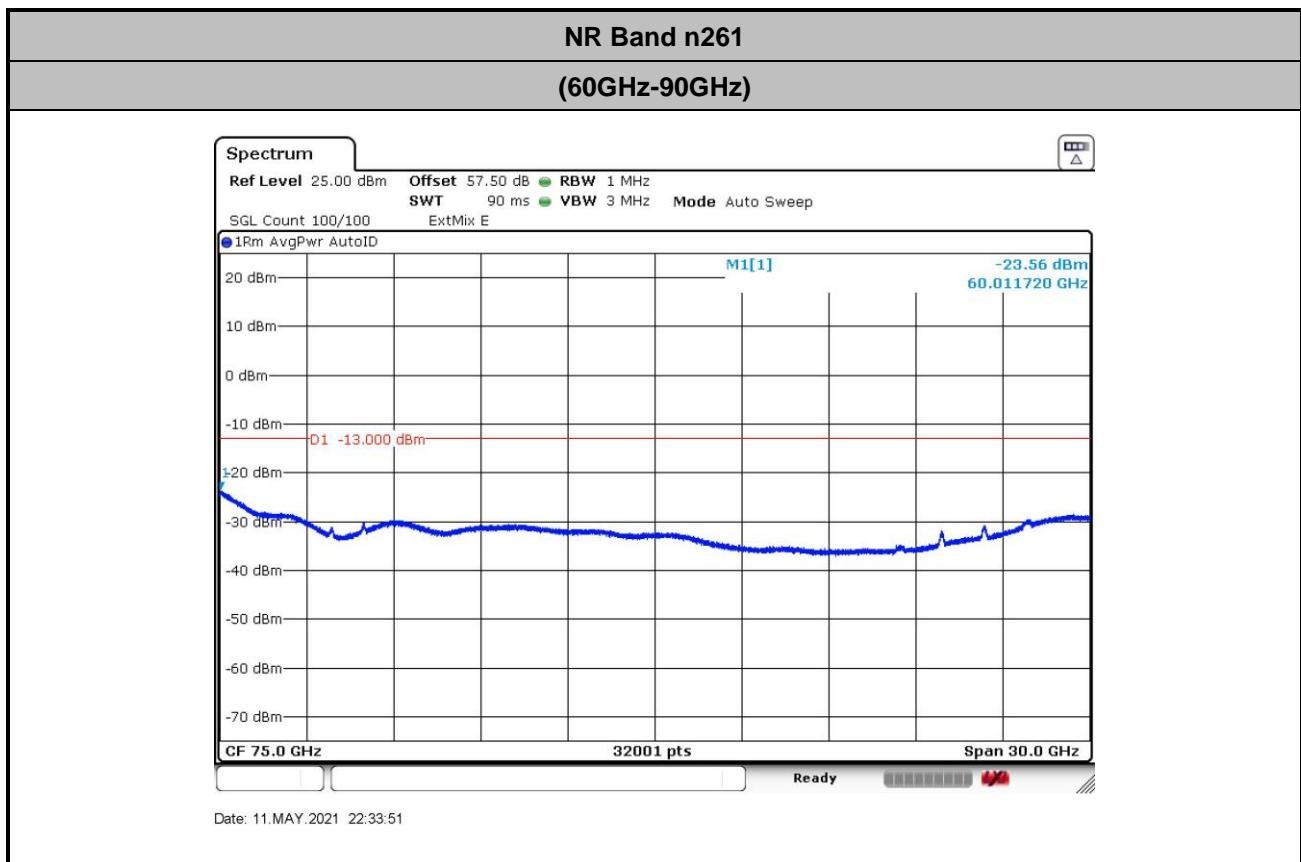
Offset = Antenna Factor (dB/m) + Cable Loss (dB) + 107 + 20log (D) - 104.8
