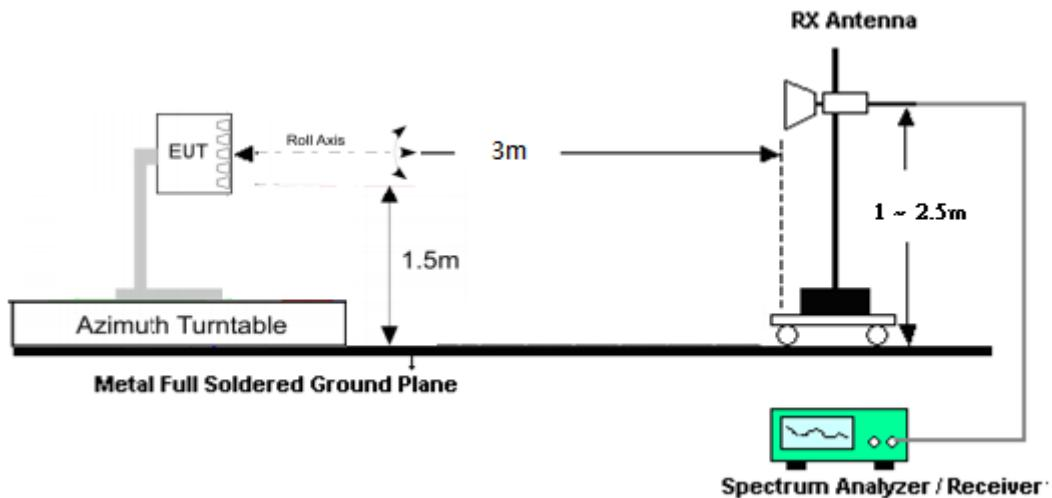
For radiated emissions above 40GHz up to 90GHz
