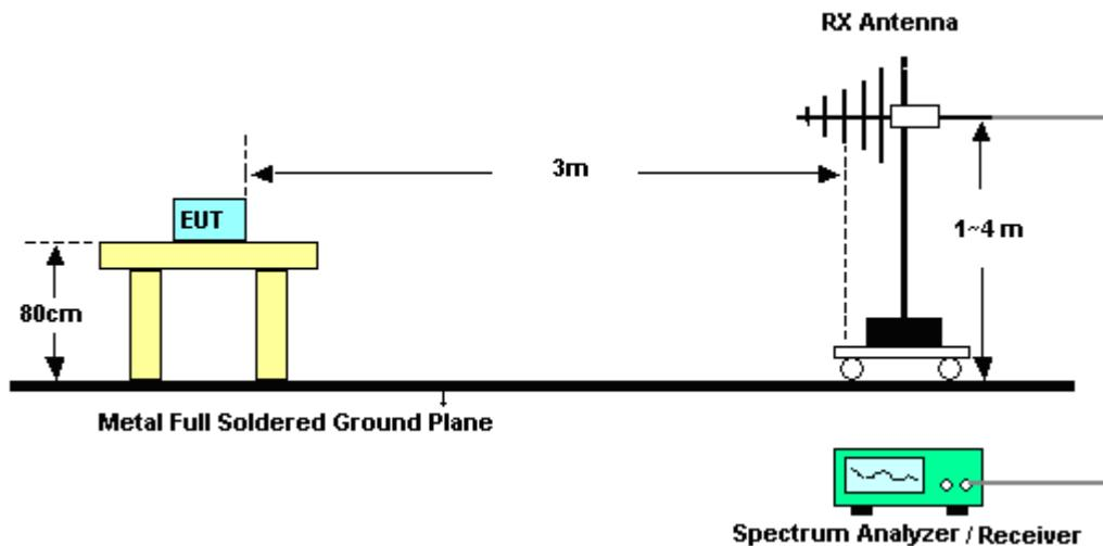
For radiated emissions 1GHz to 18GHz
