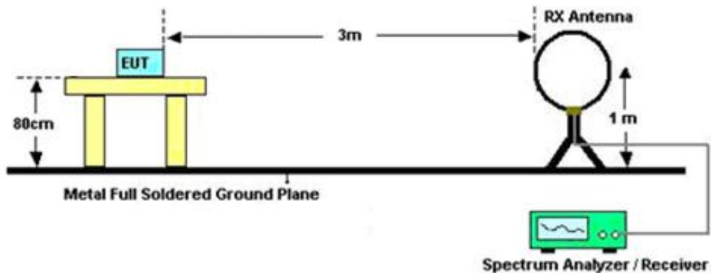
For radiated emissions from 30MHz to 1GHz
