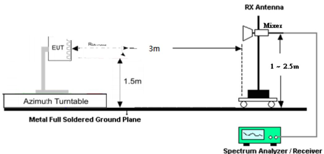
For radiated emissions above 90GHz up to 100GHz
