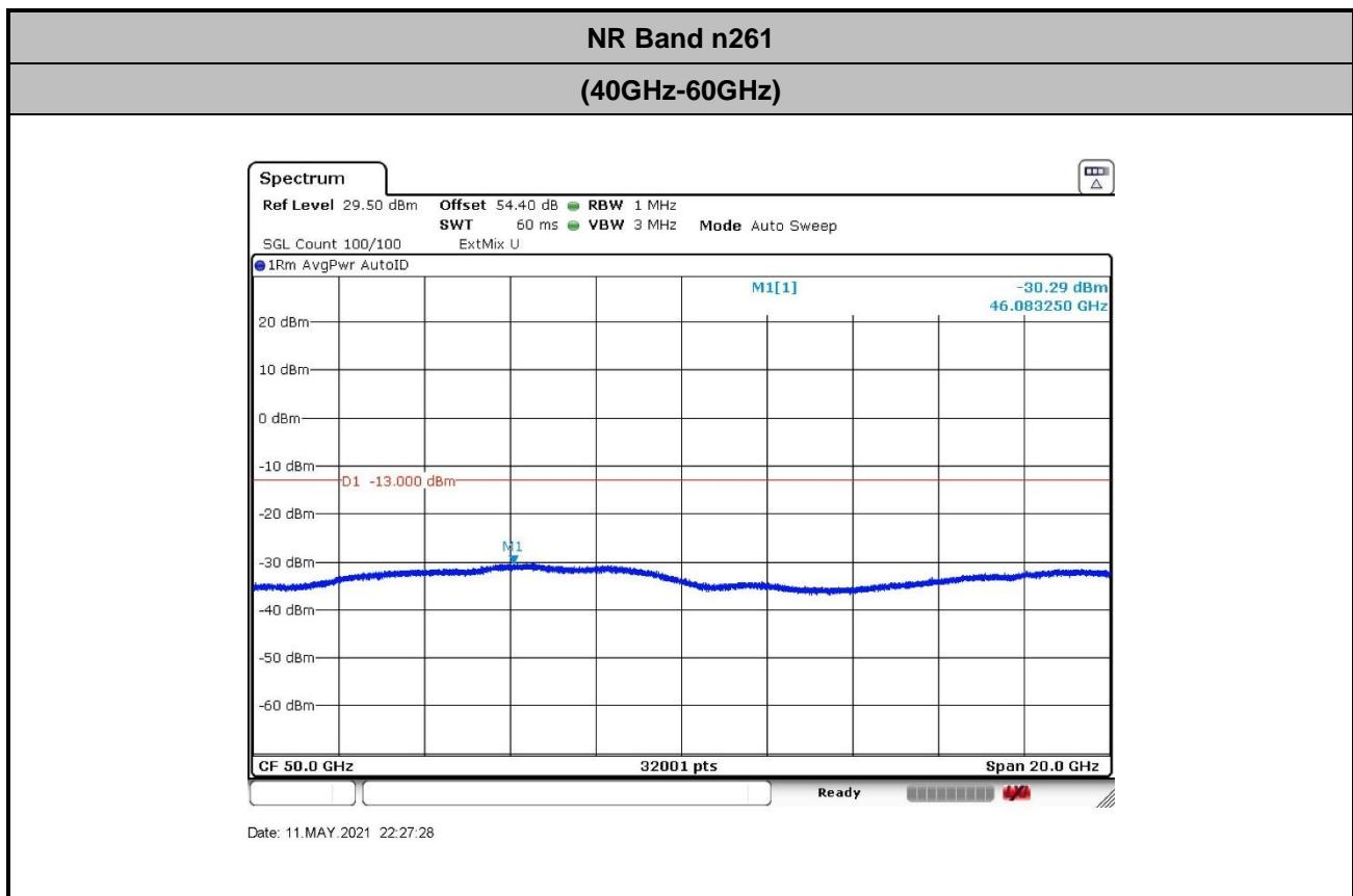
$$\begin{aligned} \text{Offset} &= \text{Antenna Factor (dB/m)} + \text{Cable Loss (dB)} + 107 + 20\log(D) - 104.8 \\ &= 42.3 + 0.34 + 107 + 20\log(3) - 104.8 = 54.4 \text{ (dB)} \end{aligned}$$
