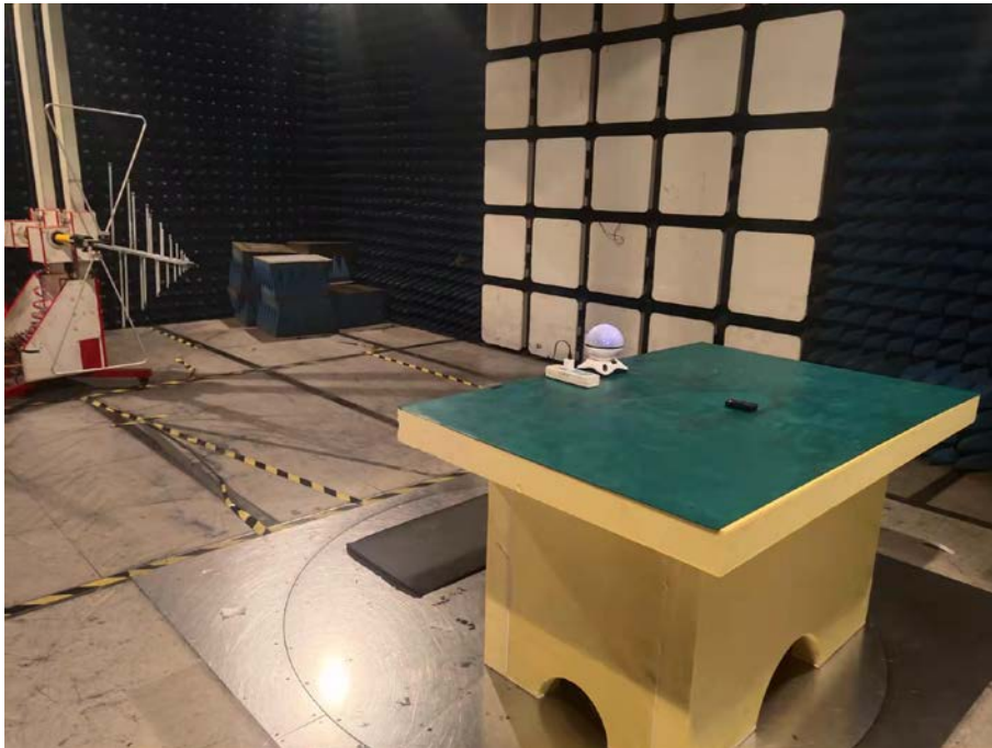
Spurious Emission Test Setup (Below 1GHz)
