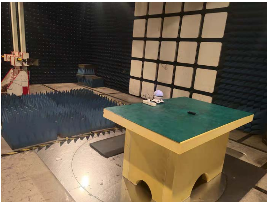
Spurious Emission Test Setup (Above 1GHz)
