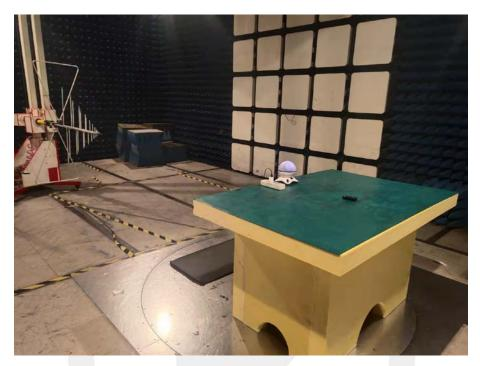
Spurious Emission Test Setup (Above 1GHz)
