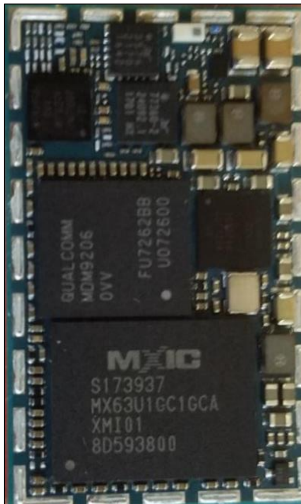
Photograph 6: Cellular module with RF Shield removed.
