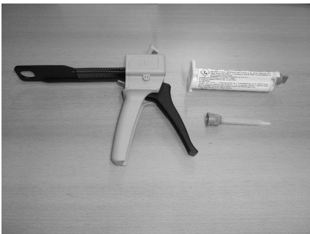
Figure 19: The three elements of the adhesive dispenser: manual applicator, two-component tube and mixing tip
