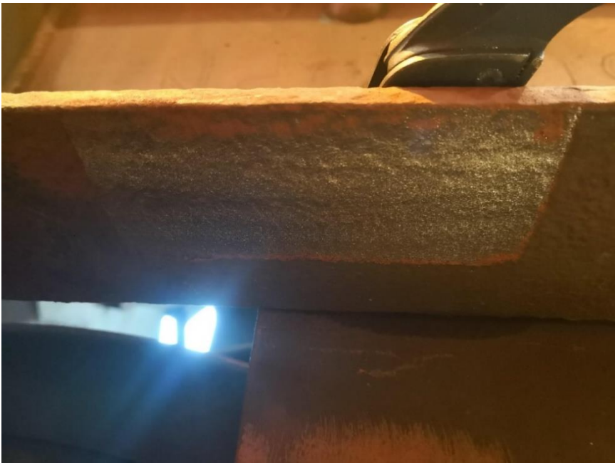
Figure 14: Example picture: stripped adhesive after using the rotary brush device (template has already been removed)
