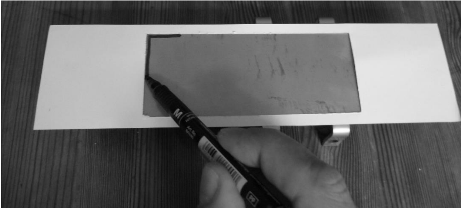
Figure 18: Mark the application area of the 2K adhesive on the back of the mounting plate using the adhesive template.
