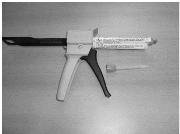
Figure 20: Step 1: Place the tube on the front of the manual applicator (pay attention to the respective piston diameters)
