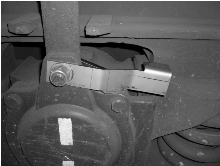
Figure 7: View of mounted reflector plate on standard wheelset bearing type Y25
