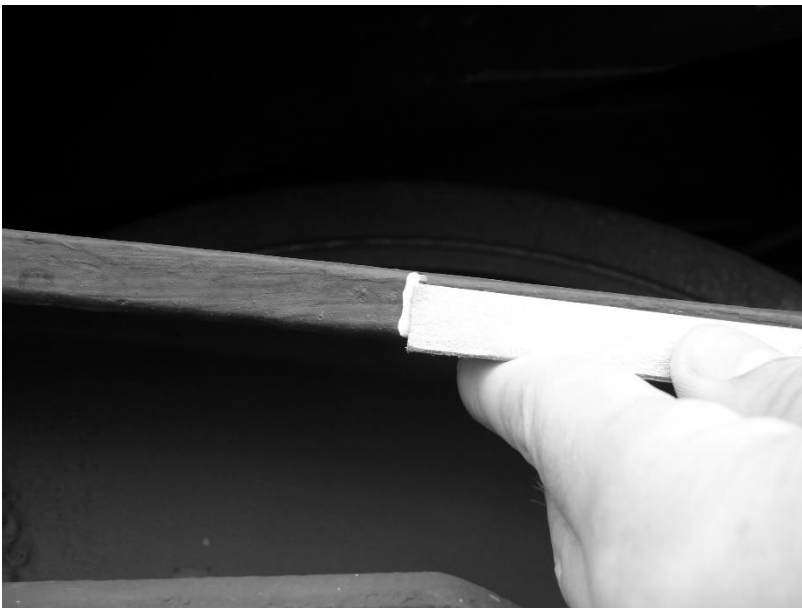
Figure 12: Apply the paint franking template to the mark known from Chapter 6.2 (the 90° bend faces the fitter).
