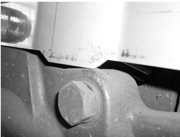
Figure 8: Correct contact of the plate widening to the axle box bearing cap
