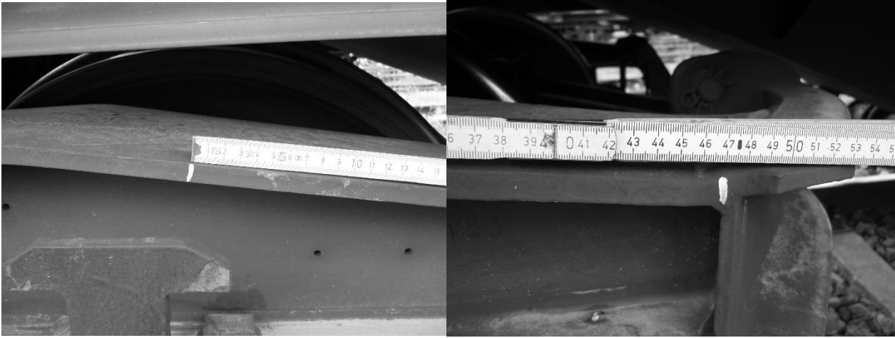
Figure 9: Measuring the Mounting Position for the Sensor and the Paint Clearance Template (Place on the right of the Head Bracket, make a mark on the left of the Mounting Plate)
