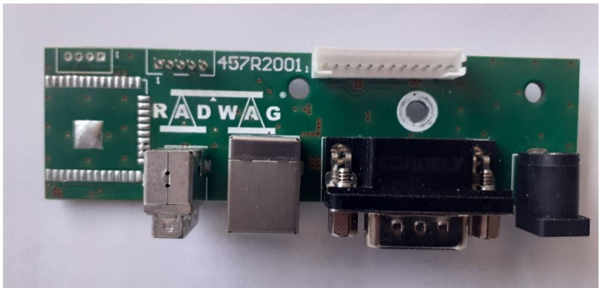
PCB 457R2001 Top view with unsoldered WiFi module
