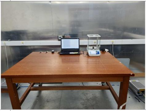
Test Setup Power Line Conducted measurement (Side area)
