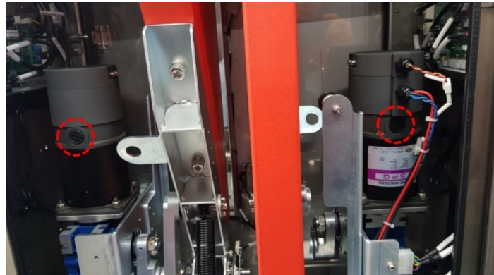
[Figure 39] DC Motor brush
