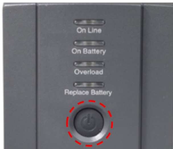
[Figure 68] UPS power switch
