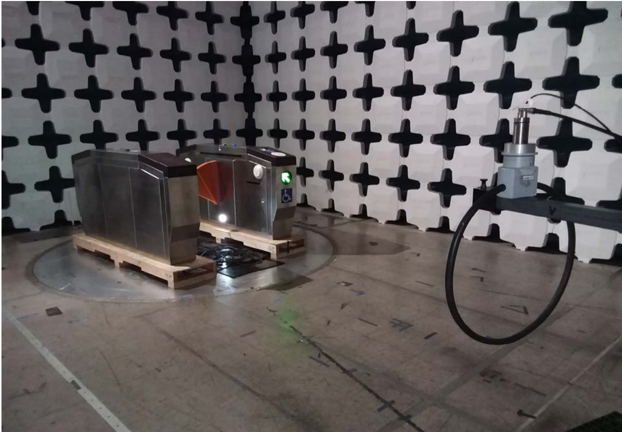
Test Configuration Photograph #1 (Radiated Emissions - Below 30 MHz)
