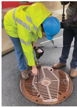
Figure 8.1 Inserting the probe into the test area.
