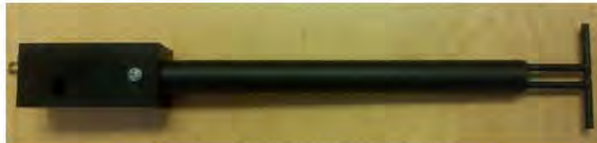
Figure 1 – MVG COMOSAR Validation Dipole
