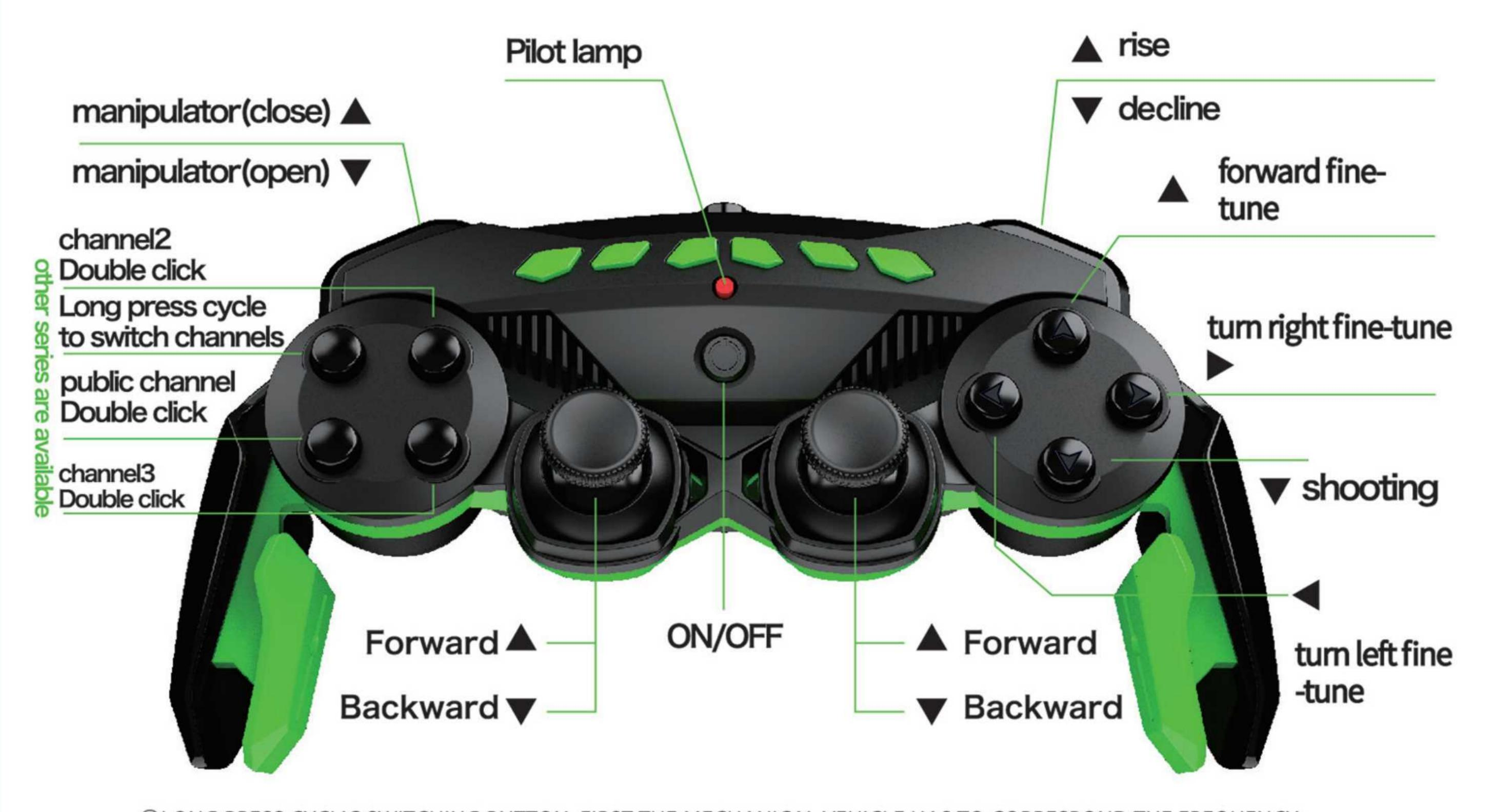
PRESS THE BUTTON TILL THE POWER LED OF THE TARGETED MECHANICAL VEHICLE LIGHTS UP AND RELEASE THE BUTTON IMMEDIATELY TO CONTROL THIS VEHICLE. KEEP PRESSING THE BUTTON TO REPEAT ABOVE-MENTIONED OPERATIONS TO SWITCH TO OTHER MODELS CYCLICALLY.
