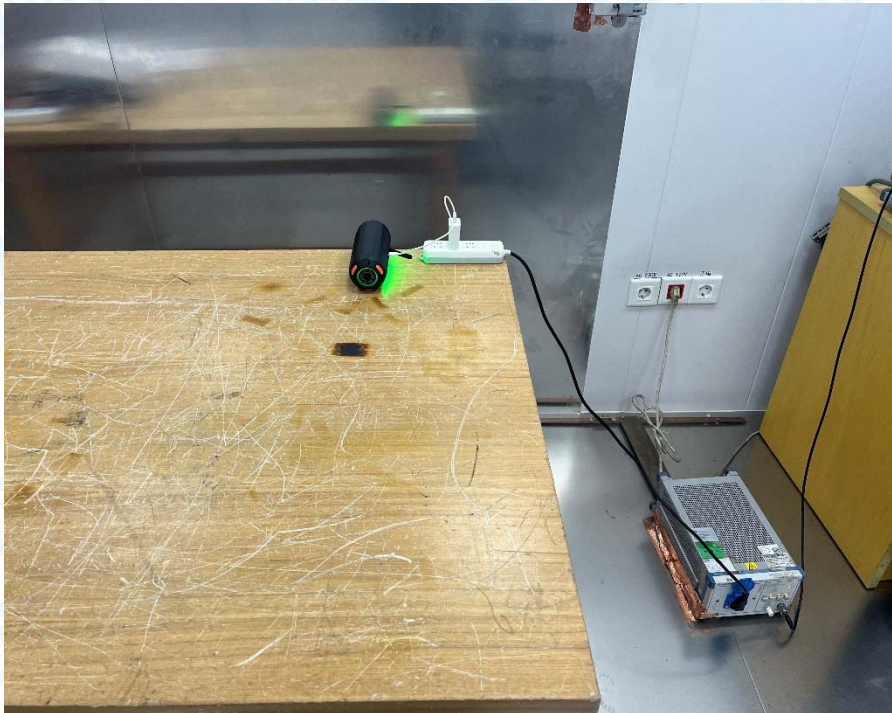
Photo of Setup for Conducted Emission
