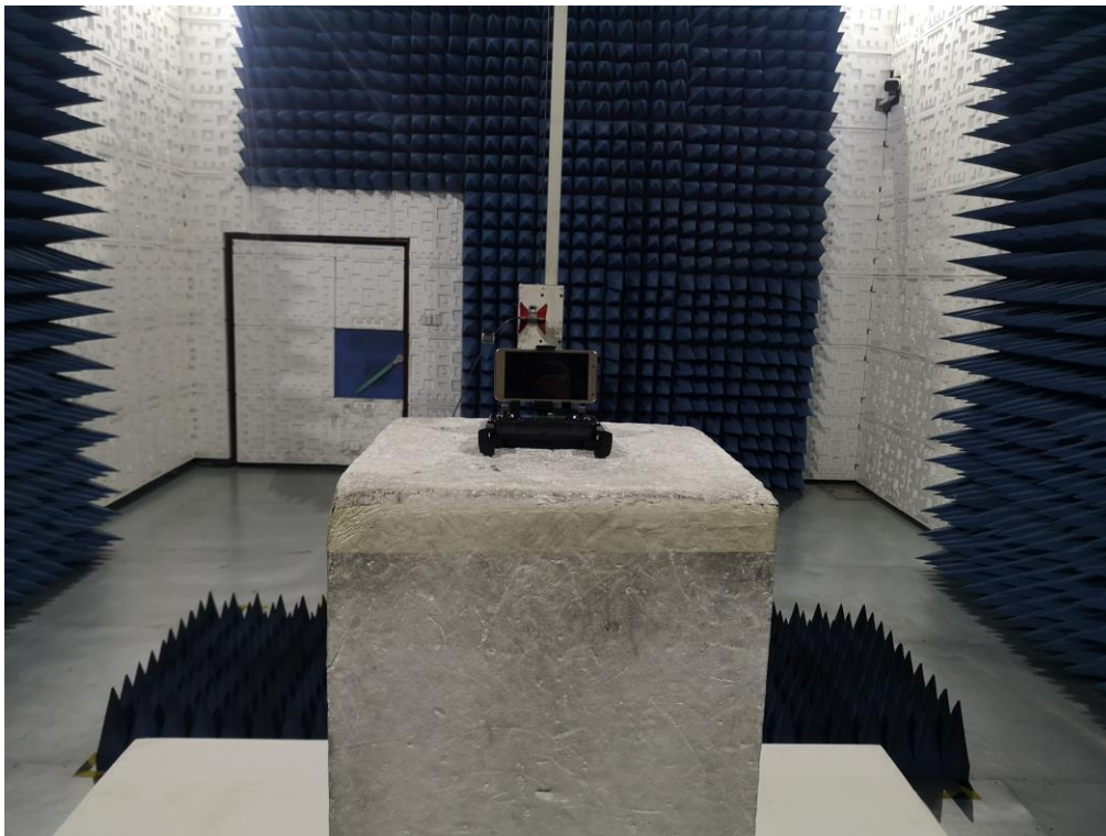
FCC RADIATED EMISSION TEST SETUP ABOVE 1
