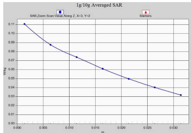
Fig. 1-18 Z-Scan at power reference point (LTE Band12)
