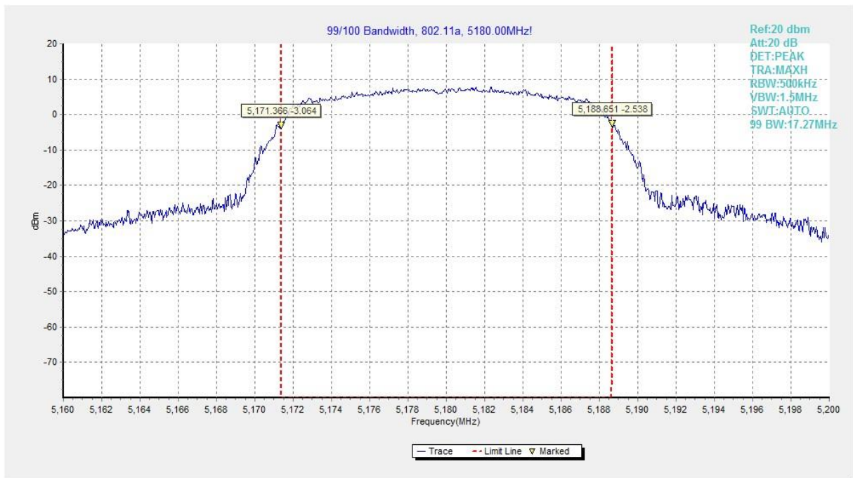
Fig.78 99% Occupied bandwidth (802.11a, 5180MHz)
