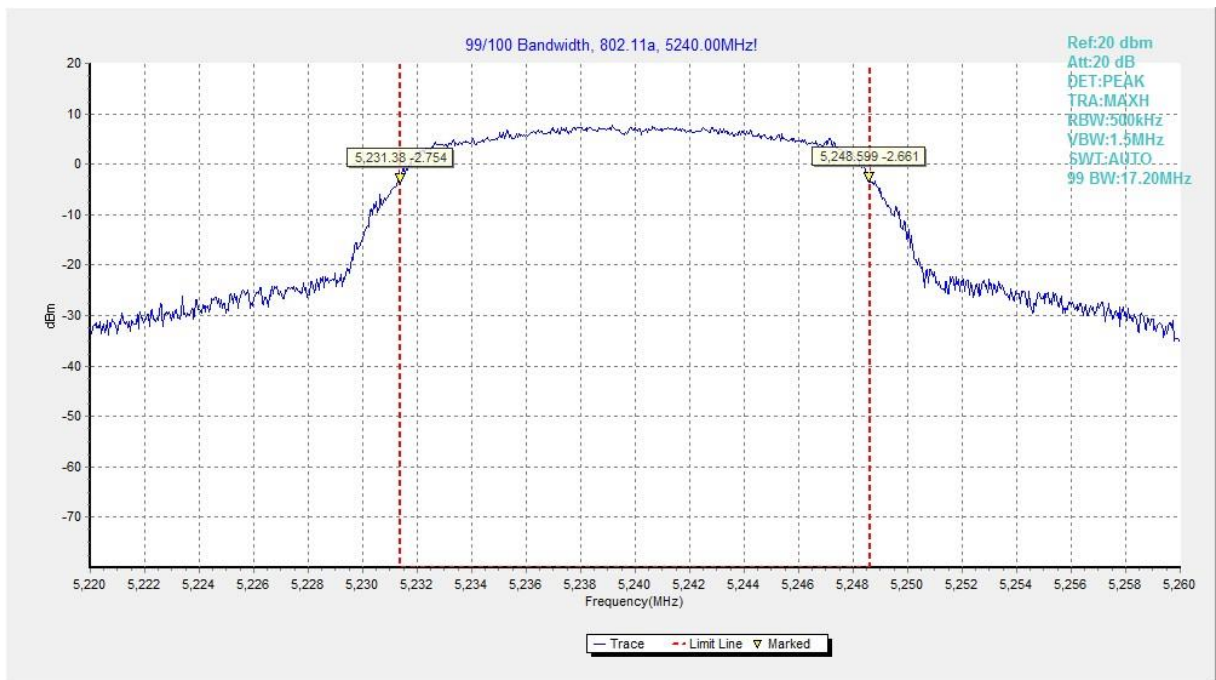
Fig.80 99% Occupied bandwidth (802.11a, 5240MHz)
