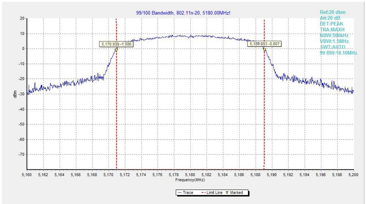
Fig.81 99% Occupied bandwidth (802.11n-HT20, 5180MHz)
