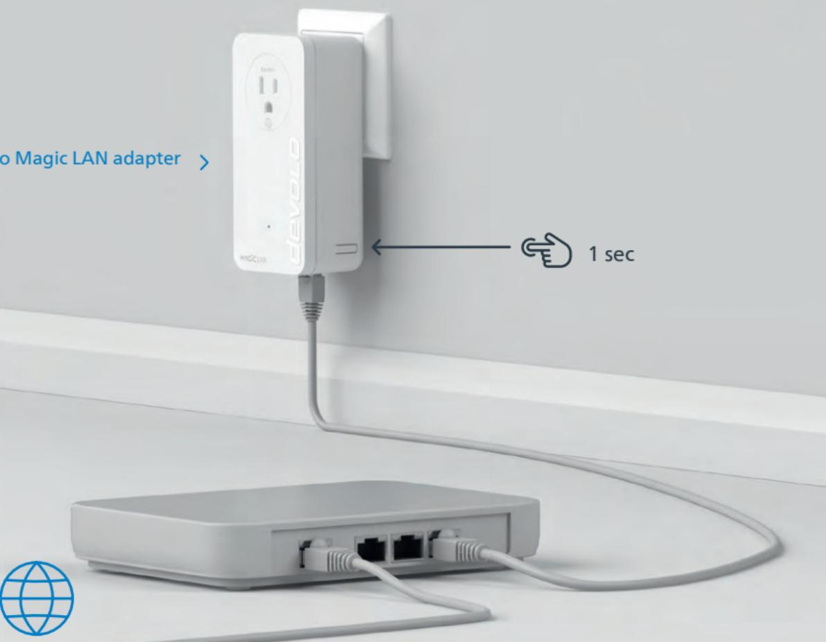
**| US |** Within 3 minutes, press the button on the side of your devolo Magic LAN adapter which is connected to the router.
