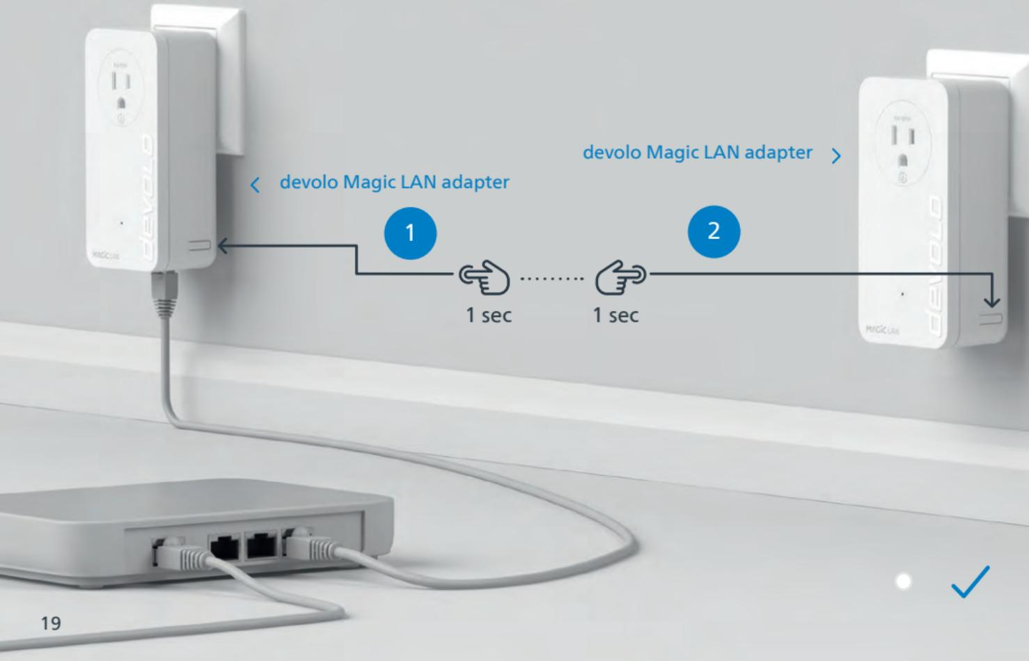
**| GB |** Within 3 minutes, press the button on the side of your devolo Magic LAN adapter, which is connected to the router. Then press the button on your second Magic LAN adapter. When all of the LEDs light up white, pairing has been completed successfully.
