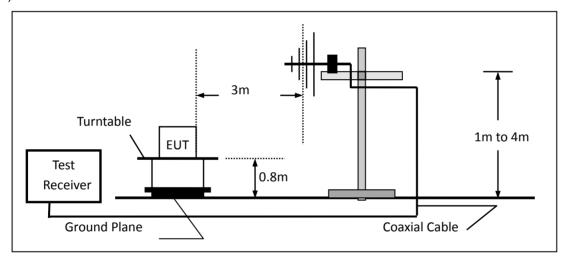
(c) For radiated emissions above 1000MHz
