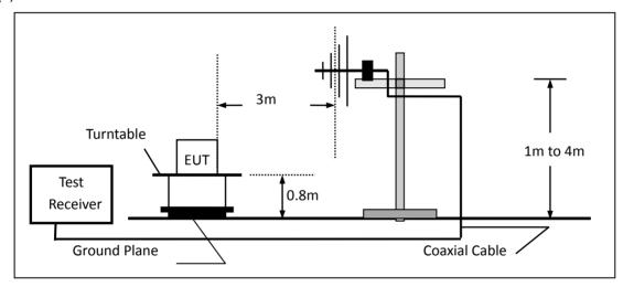
(c) For radiated emissions above 1000MHz
