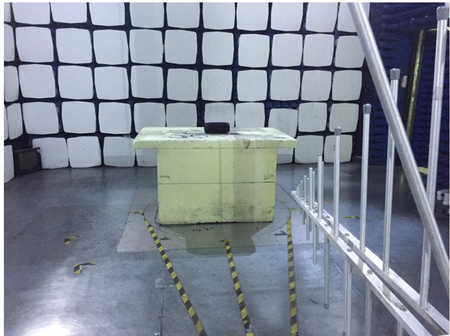
Radiation Emission Test Setup (30MHz to 1GHz)
