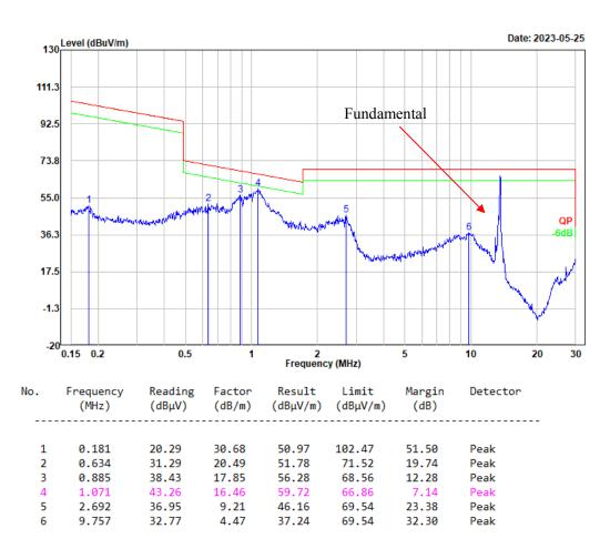
Test Mode: Transmitting Polarization: Perpendicular
