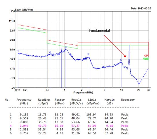
Test Mode: Transmitting Polarization: Ground-parallel
