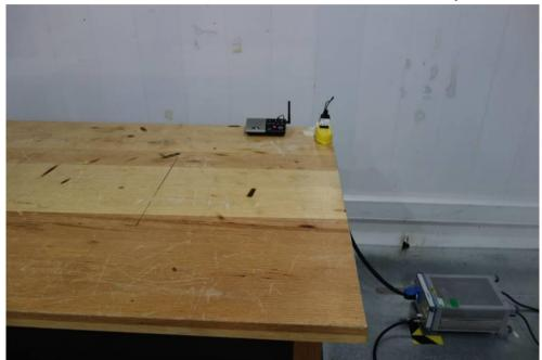
1.2 Radiated Emissions (30MHz-1GHz) Test Setup
