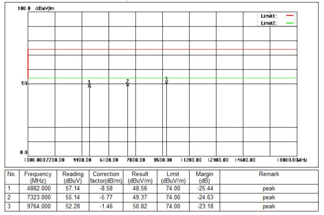
Test Mode: 01; Polarity: Vertical; Modulation:GFSK; Channel:middle
