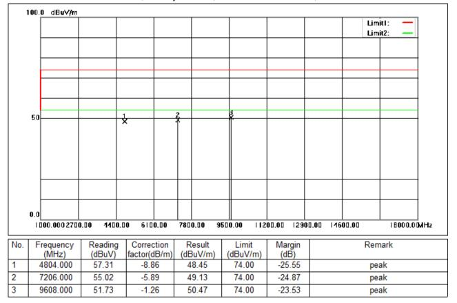
Test Mode: 01; Polarity: Vertical; Modulation:π/4 DQPSK; Channel:Low
