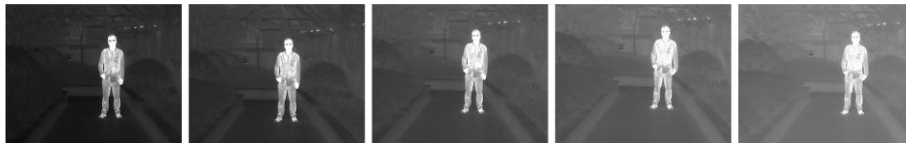
Figure 3-3 Adjust Brightness in White Hot Mode
