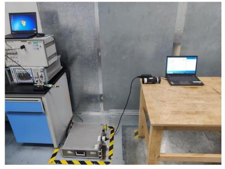
**Conducted Test Setup**
