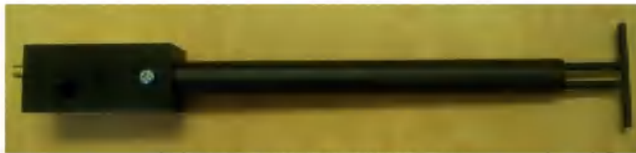
Figure 1 – MVG COMOSAR Validation Dipole
