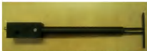
Figure 1 – MVG COMOSAR Validation Dipole
