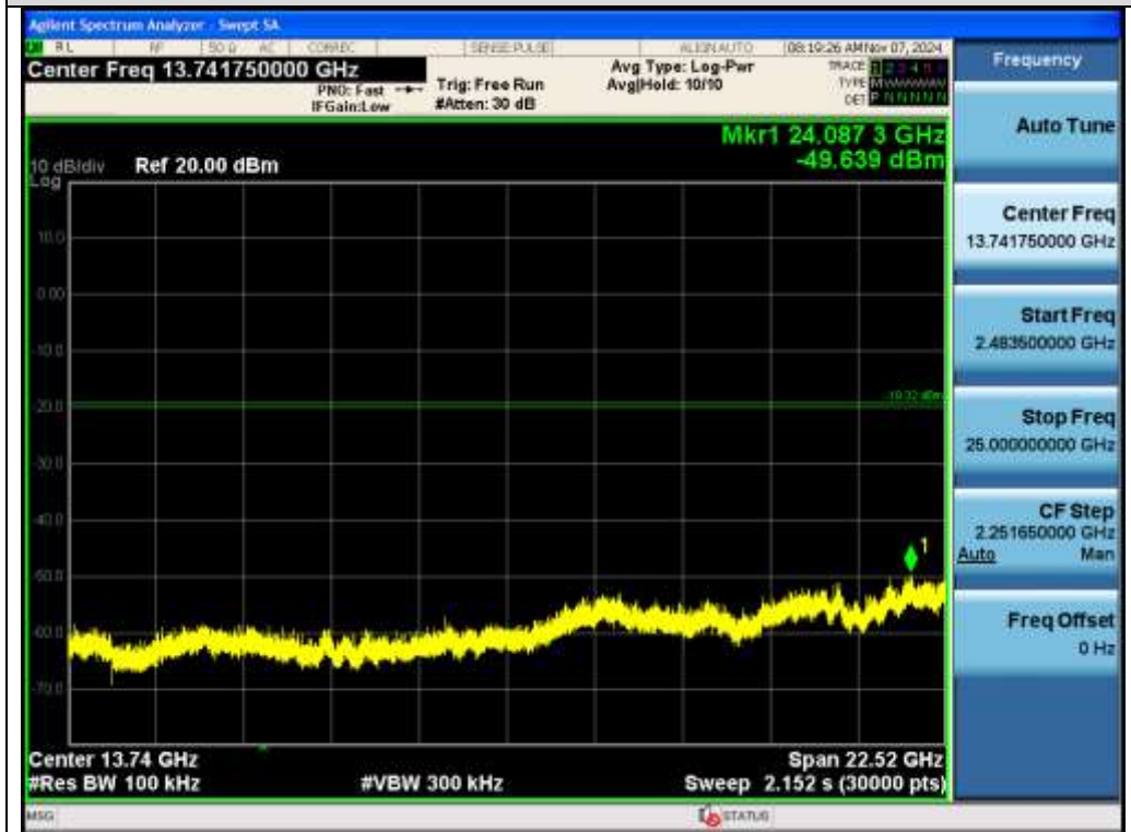
Test_Graph_EDR_ANT1_2441_3Mbps_Higher Band Emissions
