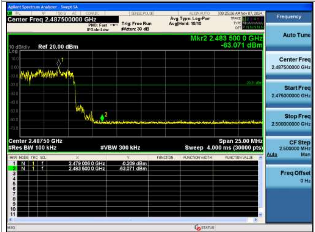
Test_Graph_EDR_HOP_ANT1_NA_3Mbps_Higher Band Edge Emissions
