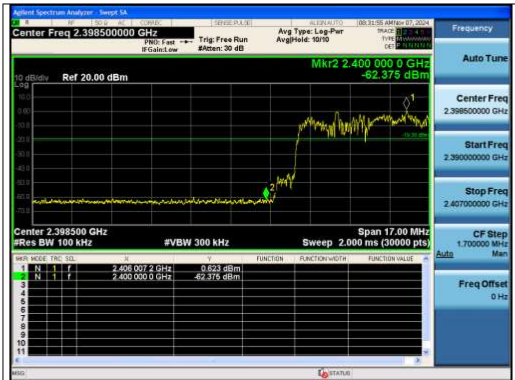
Test_Graph_EDR_HOP_ANT1_NA_2Mbps_Lower Band Edge Emissions
