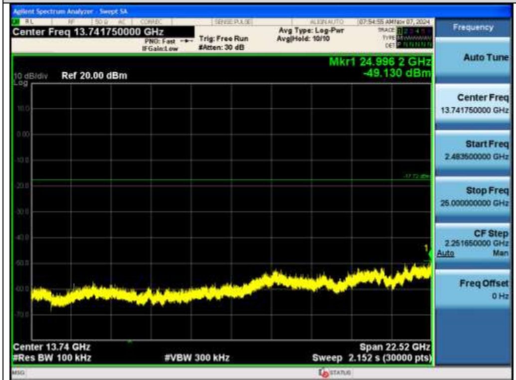
Test_Graph_BR_ANT1_2441_1Mbps_Higher Band Emissions
