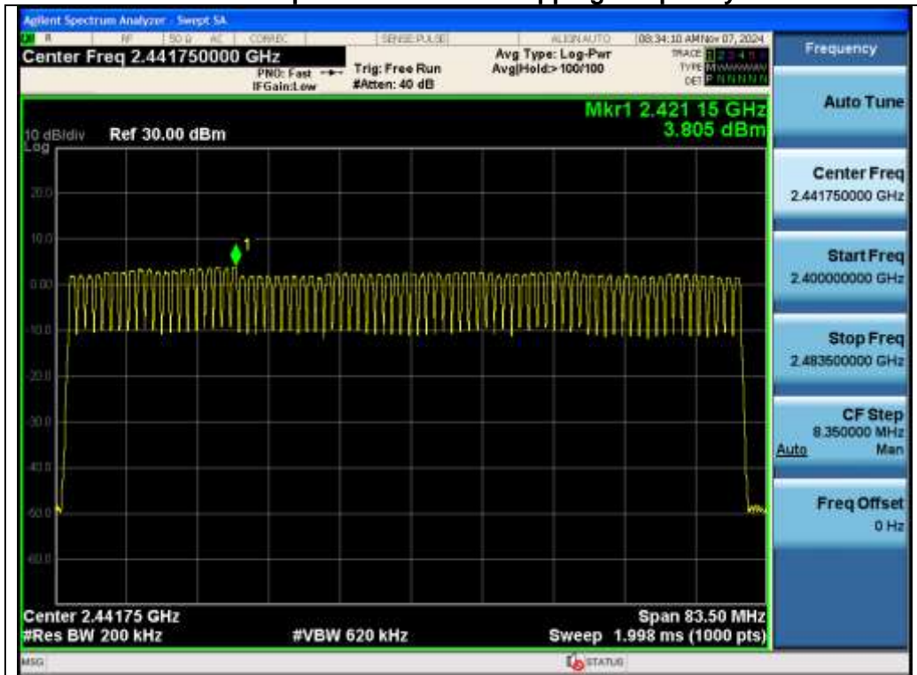
Test_Graph_BR_HOP_ANT1_NA_1Mbps_Number of Hopping
