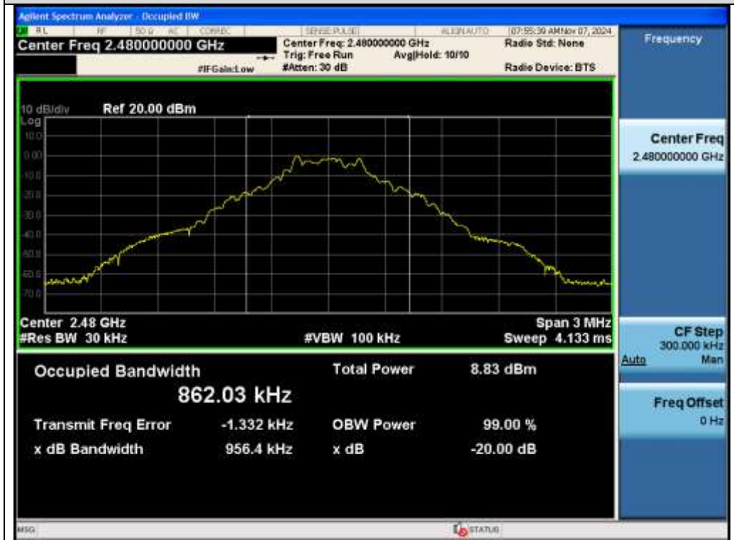
Test_Graph_BR_ANT1_2480_1Mbps_OBW
