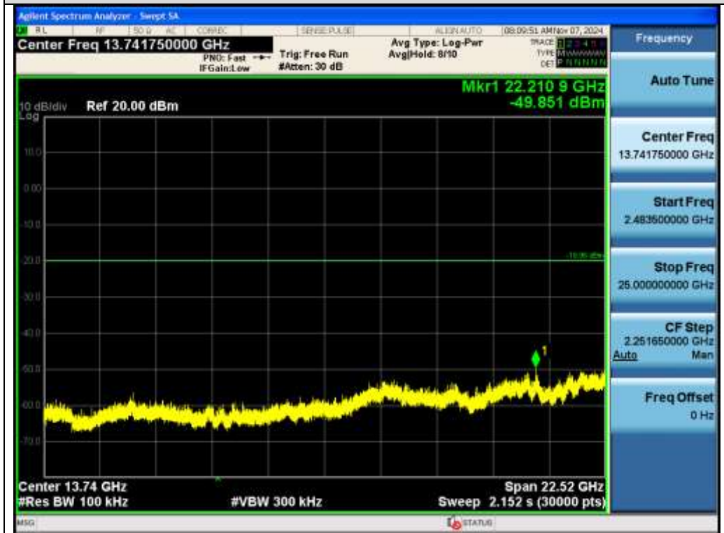
Test_Graph_EDR_ANT1_2402_2Mbps_Higher Band Emissions
