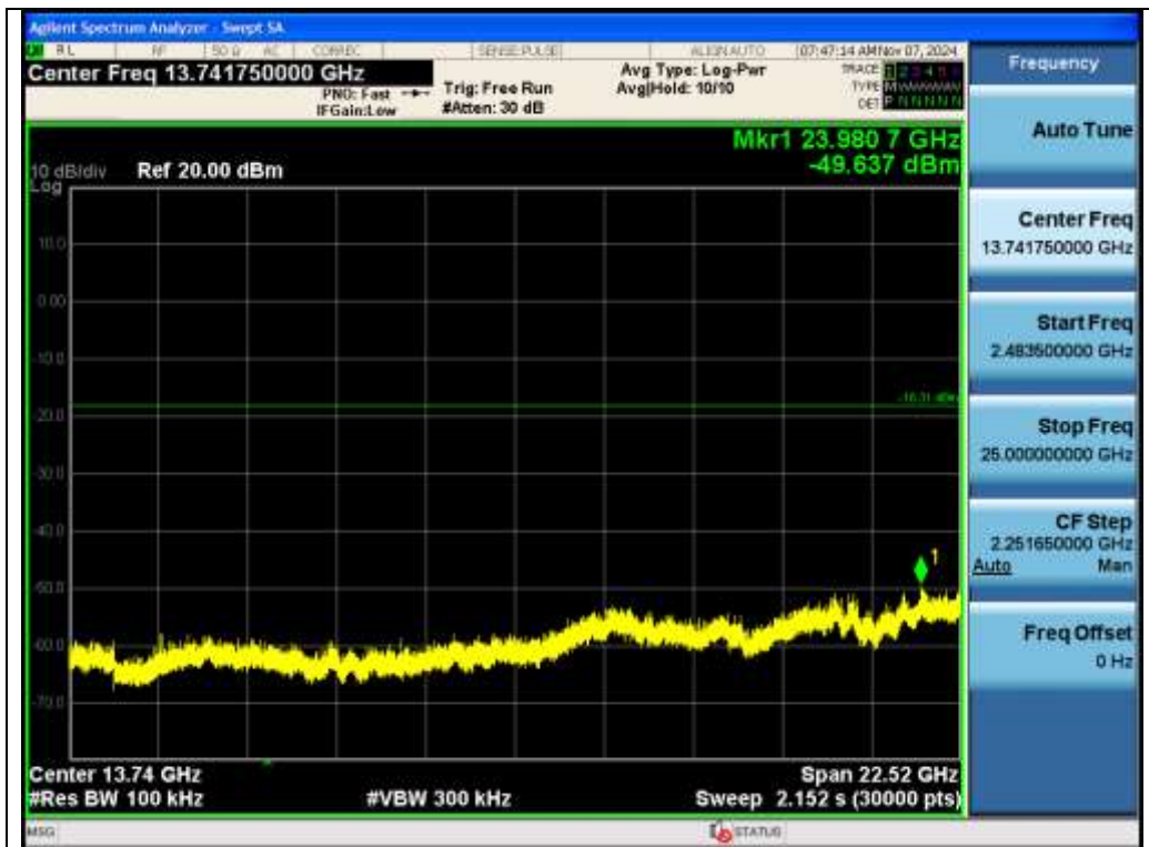
Test_Graph_BR_ANT1_2402_1Mbps_Higher Band Emissions
