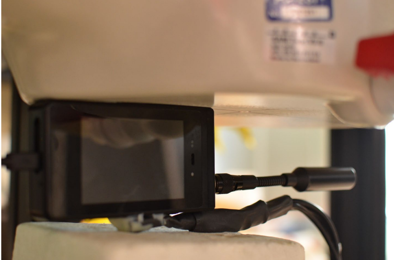
SAR Test Setup Photo 8: Extremity, Left Edge, 0 mm
