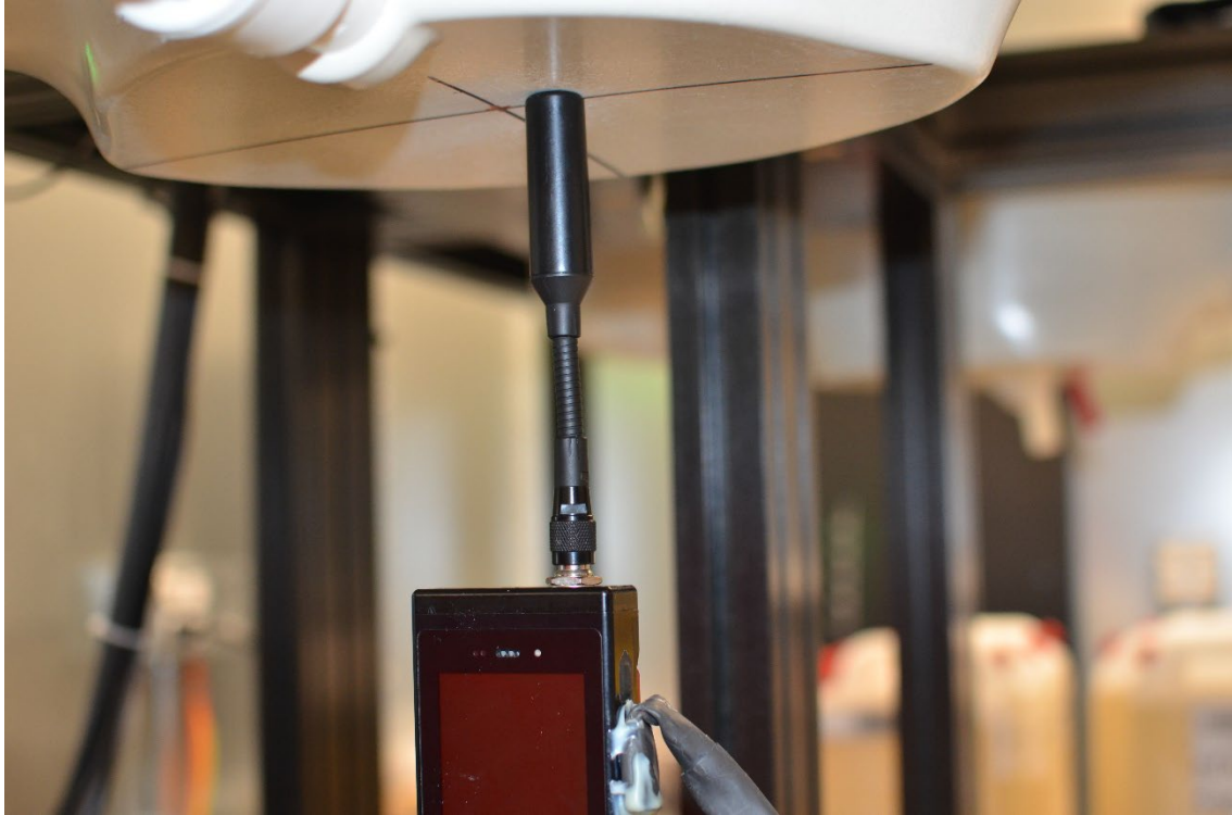
SAR Test Setup Photo 6: Extremity, Top Edge, 0 mm
