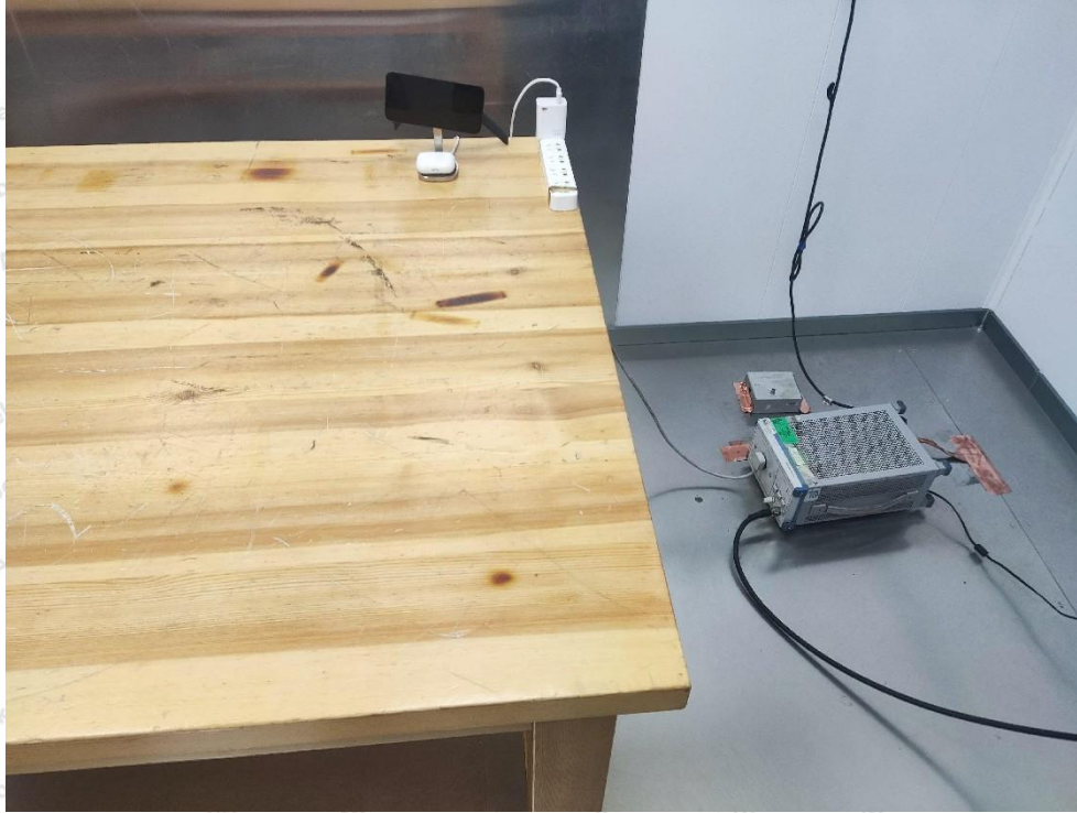
Photo of Conducted Emission Measurement
