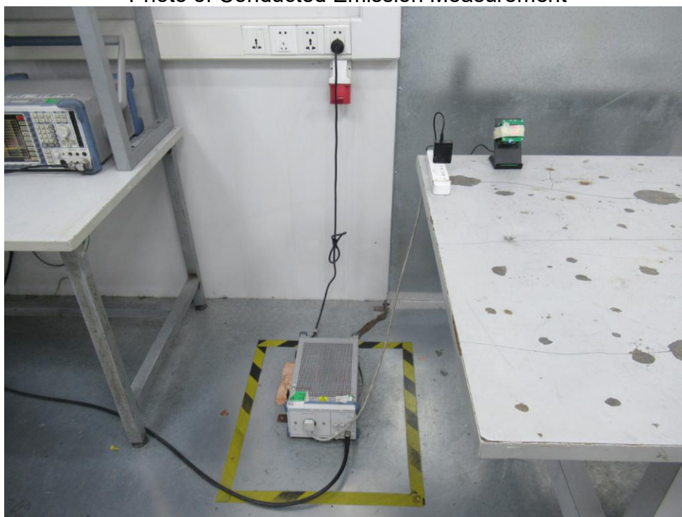
FCC ID: 2AXMG-M240 Photo of Conducted Emission Measurement
