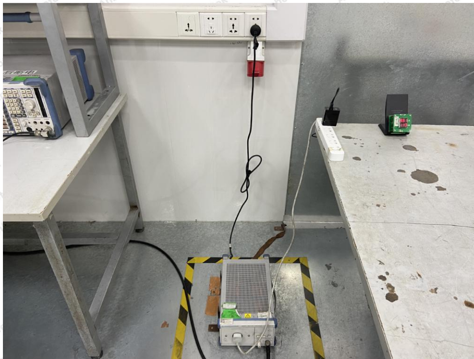
Photo of Conducted Emission Measurement
