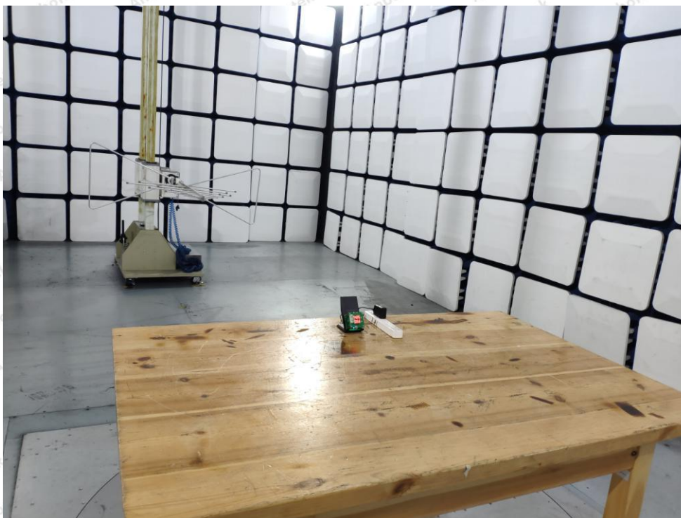
Photo of Radiation Emission Test
