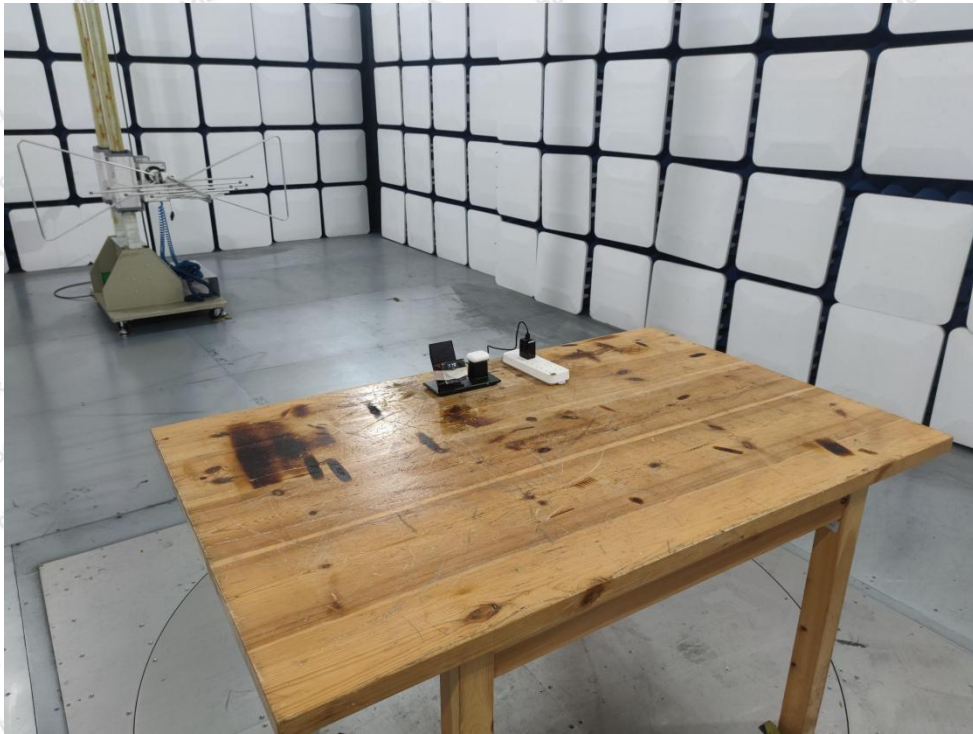
Photo of Radiation Emission Test
