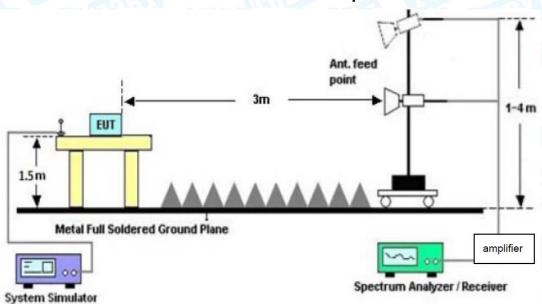
**Above 1GHz Test Setup**
