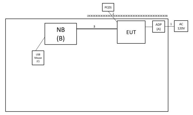
Radiated Emissions Test
