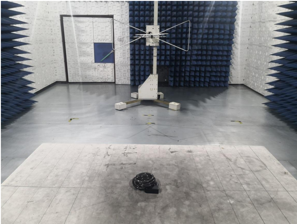
RADIATED EMISSION TEST SETUP ABOVE 1GHZ
