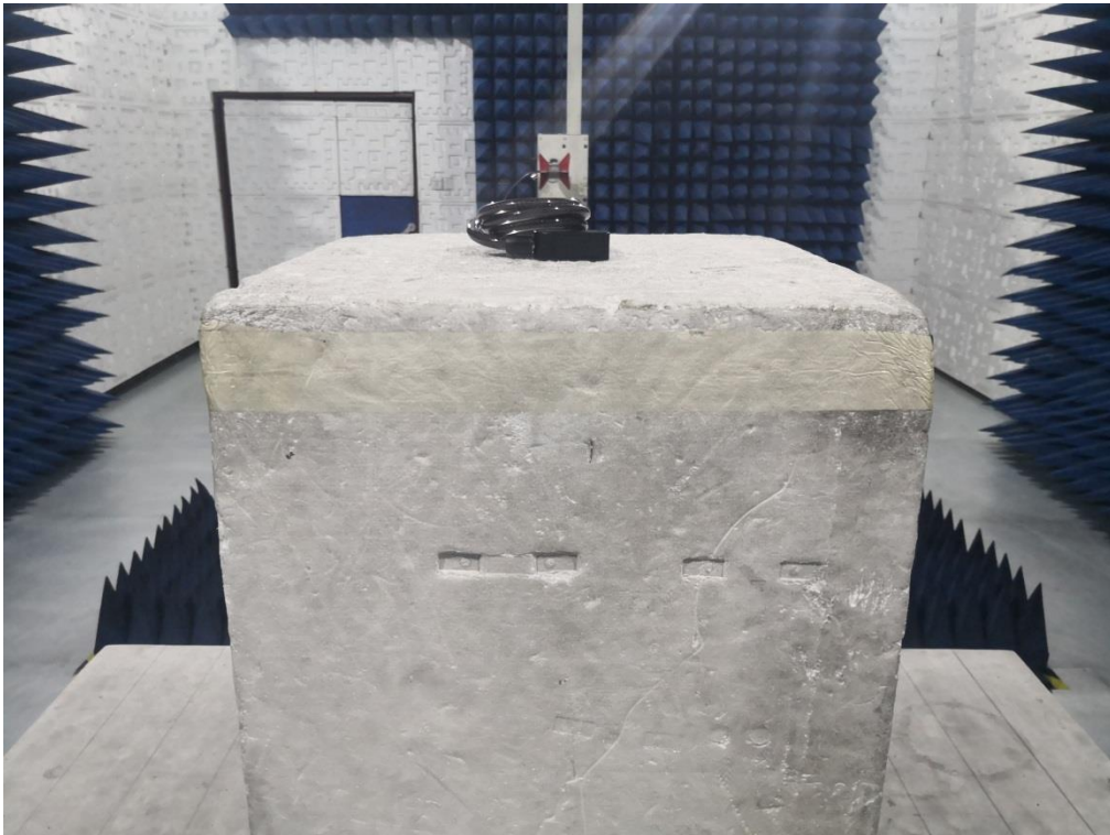
RADIATED EMISSION TEST SETUP ABOVE 1GHZ
