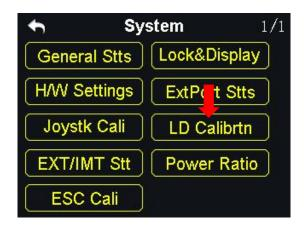
Calibrating the left dial can maintain its output accuracy. The left dial requires calibration when it stays out of the middle position (channel value is not 0) or it fails to reach the maximum / minimum position.
