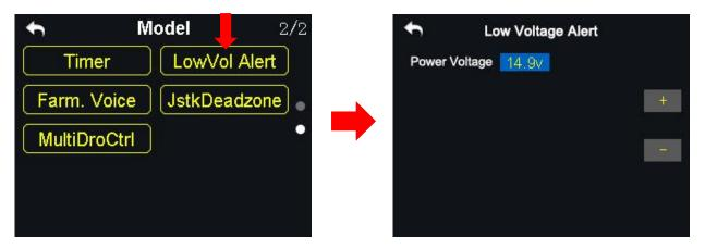
When the user's aircraft power voltage is lower than the safe level, VD32 transmitter will vibrate and send voice alert.
