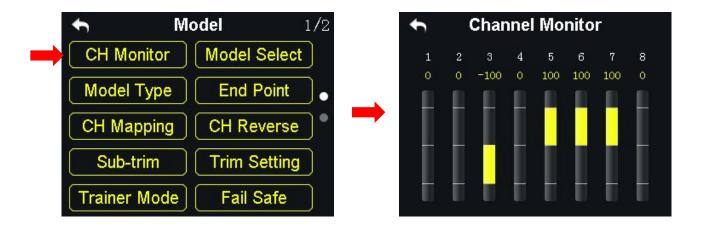
In "Channel Monitor", users can check the real-time changing of output values in all 16 channels.
