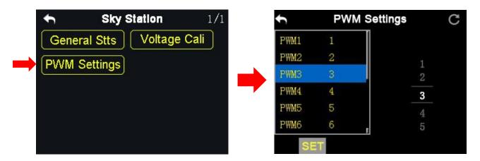
In VD32 transmitter and the PWM mode, users can redefine the output channel of the sky station (channel 1-9 in default), so that if the channel 9 is already working in SBUS or PPM mode, the PWM ports 1 to 8 can still output to the channels 1 to
