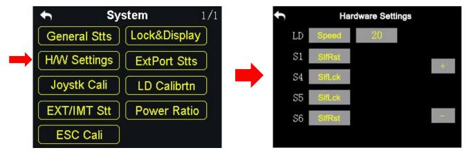
Through the H / W settings users can do advanced settings for the left dial (LD) to switch it between the Position Mode and the Speed Mode and the switch S1 / S4 / S5 / S6 to switch between Self-locking and Self-resetting.
