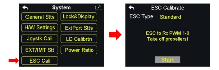
VD32 transmitter simplified the ESC calibration a lot. Users just connect their ESC to VD32 receiver's PWM port 1 to 8, then follow the tips in the screen menu or the steps below to finish calibration.
