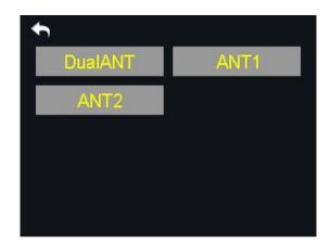
Both the transmitter and the sky station have two antennas. Users can decide which antenna to use, the antenna 1, the antenna 2 or both according to their requirement.
