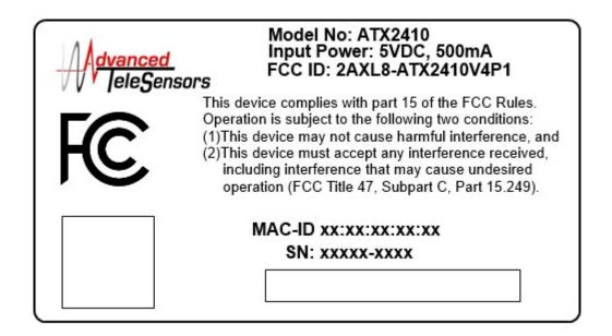
The Square on the left side (as you view the label) will contain a QR Code with MAC ID and Serial number of this device. The rectangular area in the bottom-center will contain a barcode of the Serial Number of this device. The label would be placed on the back of the enclosure as indicated. The size of the label is 2-3/8" x 1-1/4".
