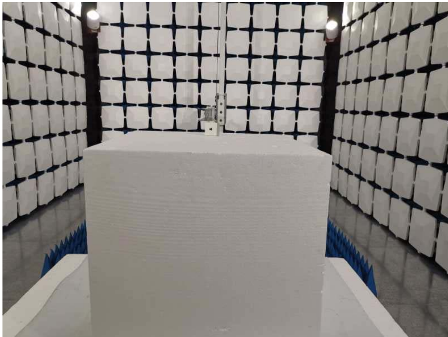
Above 1GHz for radiated emission test setup
