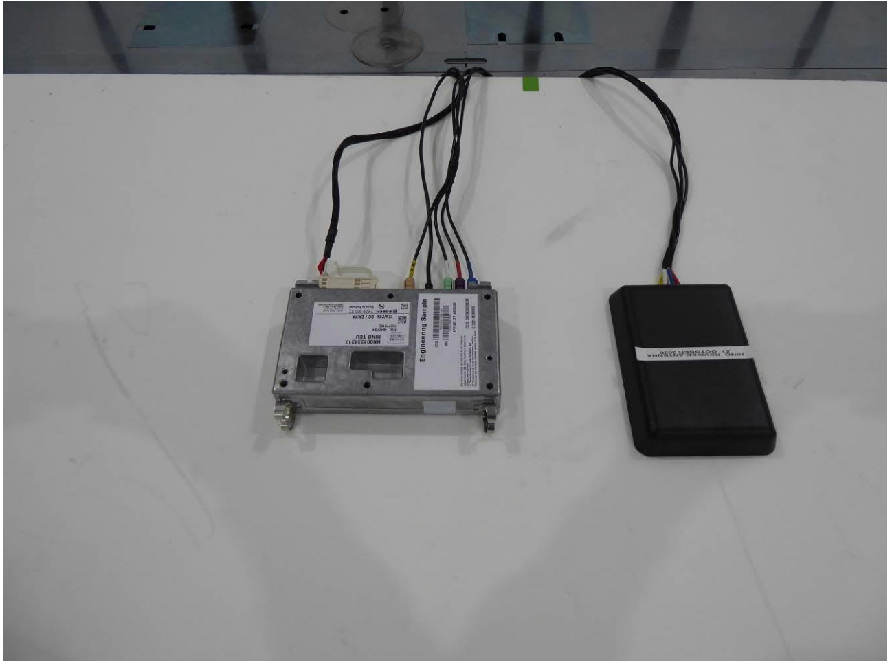
Test setup – radiated test in semi-anechoic chamber (M276)
