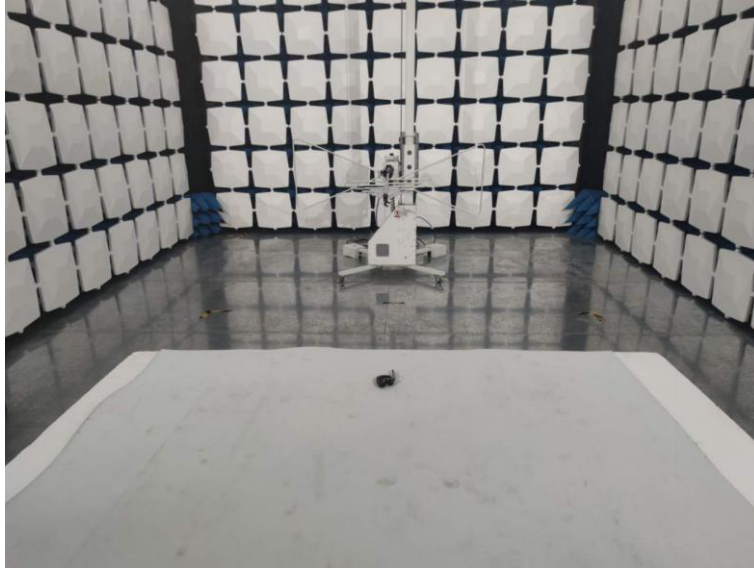
Blow 1GHz for radiated emission test setup
