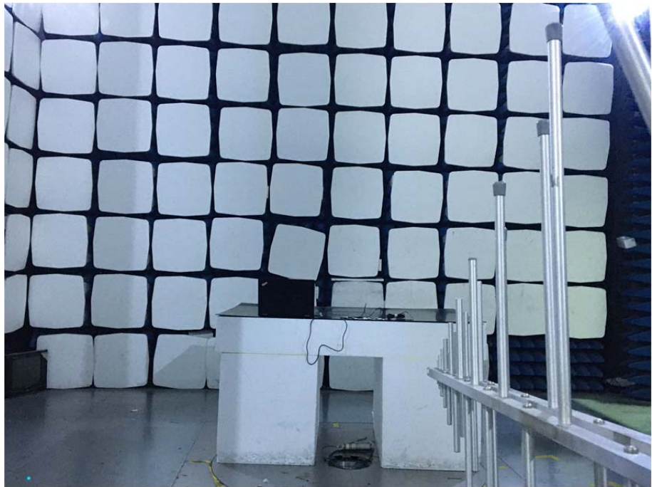
Radiation Emission Test Setup (30MHz to 1GHz)
