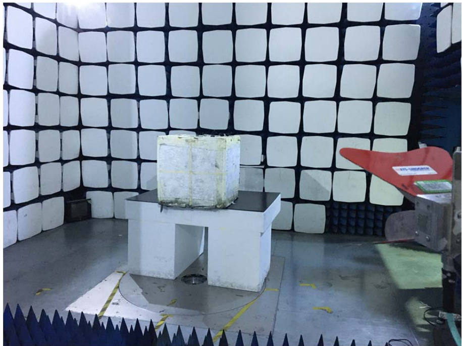
Radiation Emission Test Setup (1GHz to 18GHz)
