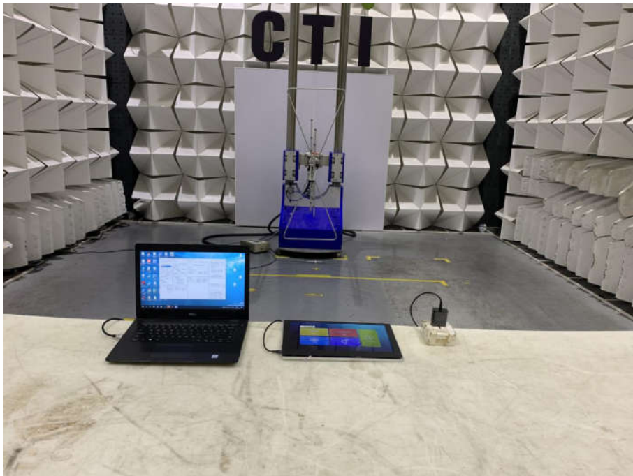
Radiated spurious emission Test Setup-2(Below 1GHz)
