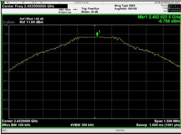
GFSK on Channel 39
