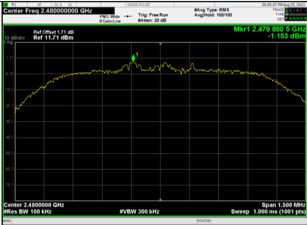
\pi/4 -DQPSK on Channel 78
