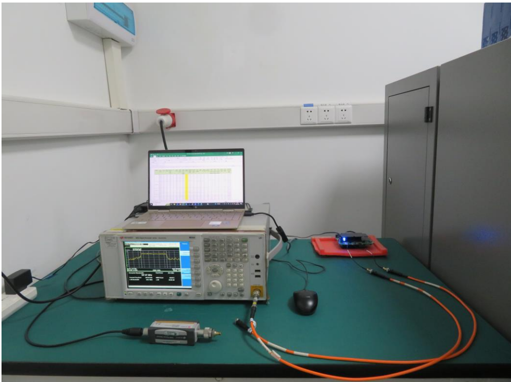
Description: Conducted Test Setup
