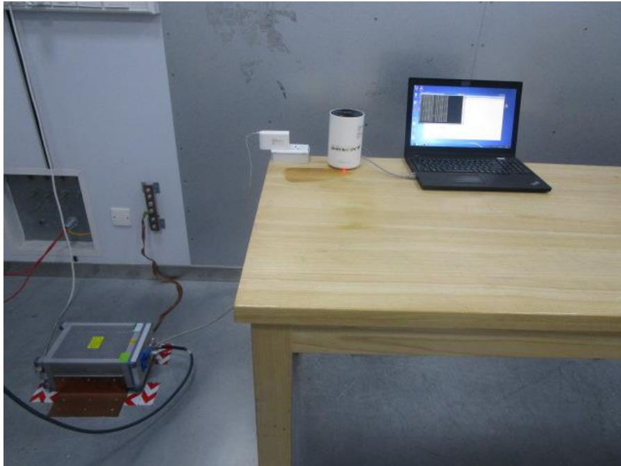
POWERLINE CONDUCTED EMISSIONS MEASUREMENT SETUP
