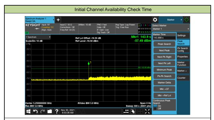
Note: The EUT does not transmit any beacon or data transmissions until at least 1 minute after the completion of the power-on cycle (83.9sec). Initial beacons/data transmissions are indicated by marker 1 (143.9 sec).
