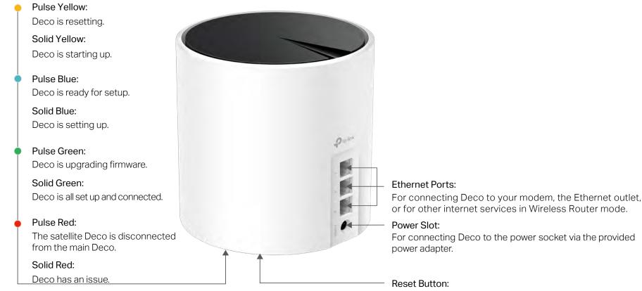
Press for 1 second and release to reset Deco to factory default settings. The light changing from pulsing yellow to solid yellow indicates a successful reset.
