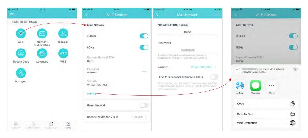
Set channel width for 5GHz Wi-Fi. 160MHz provides better Wi-Fi performance.
