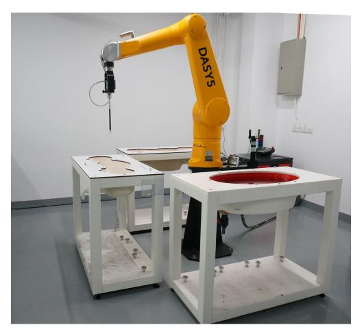
Liquid depth in the flat Phantom (≥15cm depth)
