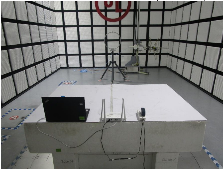
RADIATED RF MEASUREMENT SETUP (Below 30MHz)
