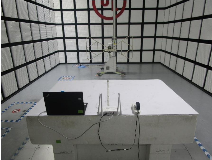
RADIATED RF MEASUREMENT SETUP (Below 30MHz)
