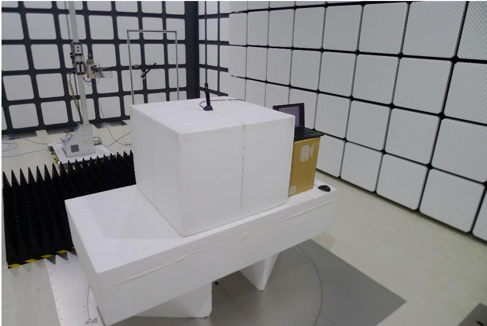
Description: Radiated Emission Test Setup for 18GHz~40GHz
